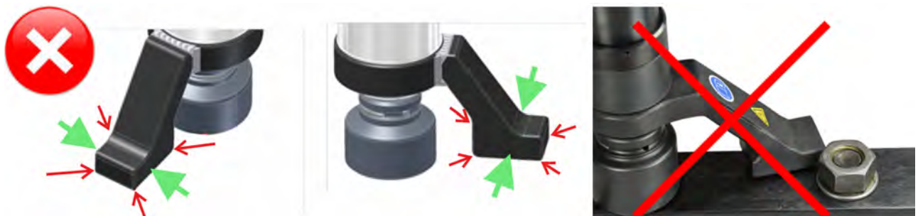
Fig. 20: Reaction arm braced incorrectly
