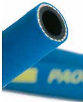
Rubber hoses with textile braid reinforcement; externally with textile effect for an easier grip; excellent resistance to oil and abrasion; blue coloured; working pressure: 20 bar - 290 psi. Suggested for 1" e 3/4" impact wrenches. Length on demand.
