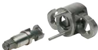
The twin-hammer system produces a double impact for each cycle on both sides of the shaft. The use of 2 opposite hammers allows to obtain a balanced impact. It is mainly used for 1/2 inch impact wrenches.
