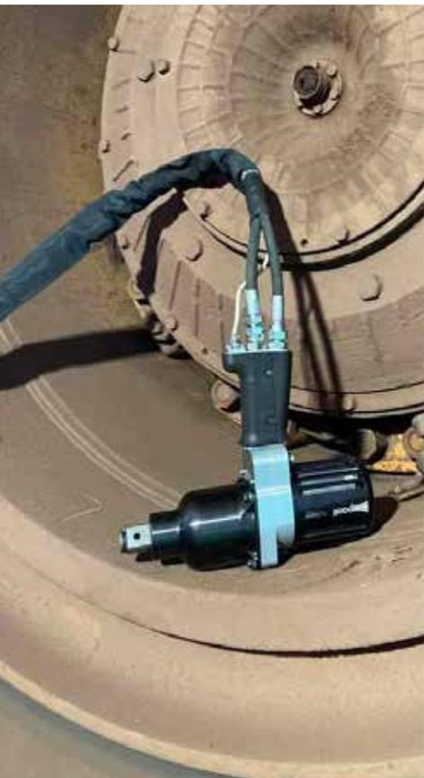
Paoli electro-hydraulic impact wrenches are equipped with an economic and ecological system: you consume energy only when you use the impact wrench. The hydraulic mechanism also allows torque repeatability and higher torque compared to pneumatic models of equal weight.
