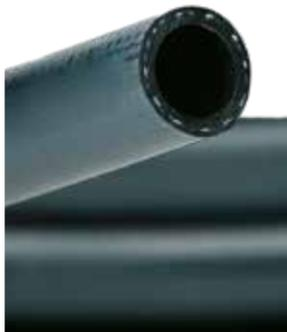
Polyurethane hoses extremely flexible and light; spark proof, ideal for light devices; black coloured; working pressure: 10 bar - 145 psi. Suggested for 3/8" e 1/2" impact wrenches. Length on demand.
