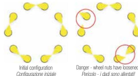
Dustite LR (long reach) combines a nut loosening indicator and a dust cap. Dustite LR is designed specifically for use on vehicle wheels with trims.
