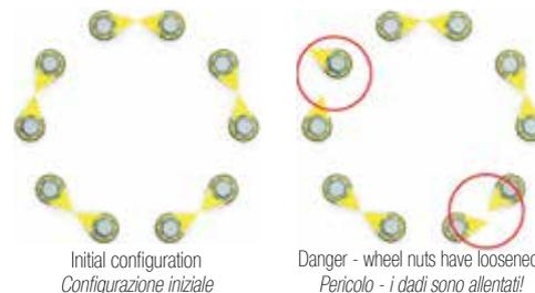
Dustite combines a nut loosening indicator and a dust cap which helps to protect the nut.
