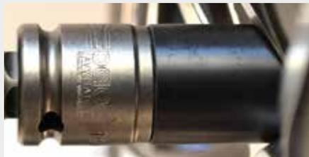
**paoli** impact sockets for alloy wheels application allow not to damage the wheel as they have a black teflon part (detached from the metal socket) that can rotate. This feature enables the tyre repairer to work with no worries and avoid marking or scratching the wheel, also in the presence of grains of dust that in the rotation of the socket could damage the wheel.
