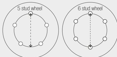
How to measure the pitch circle diameter (PCD)
