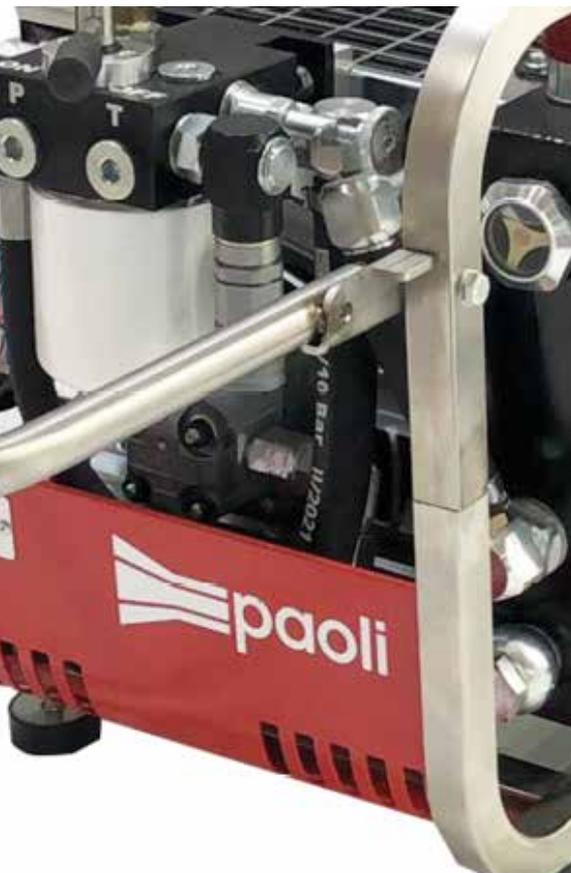
DYNO-M GASOLINE micro power pack with 6 Hp gasoline engine – recoil start is designed to guarantee the minimum weight and easy transportability. The machine is available in two configurations of hydraulic power: 20 L/min @ 95 Bar or 12 L/min @ 160 Bar.
